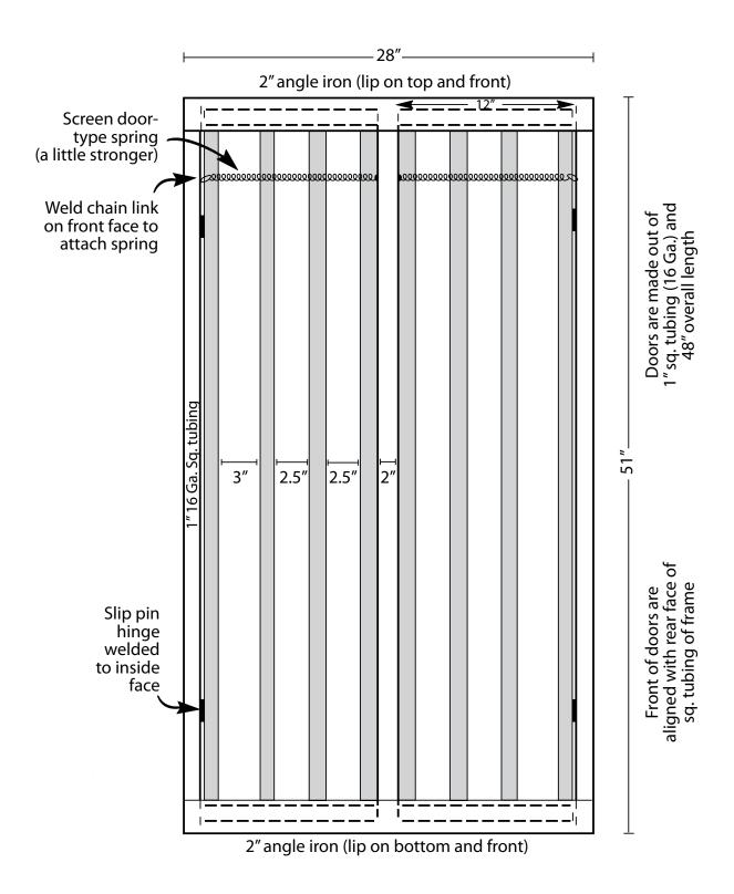
Specifications needed for the construction of a double spring door or saloon-style trap door.
