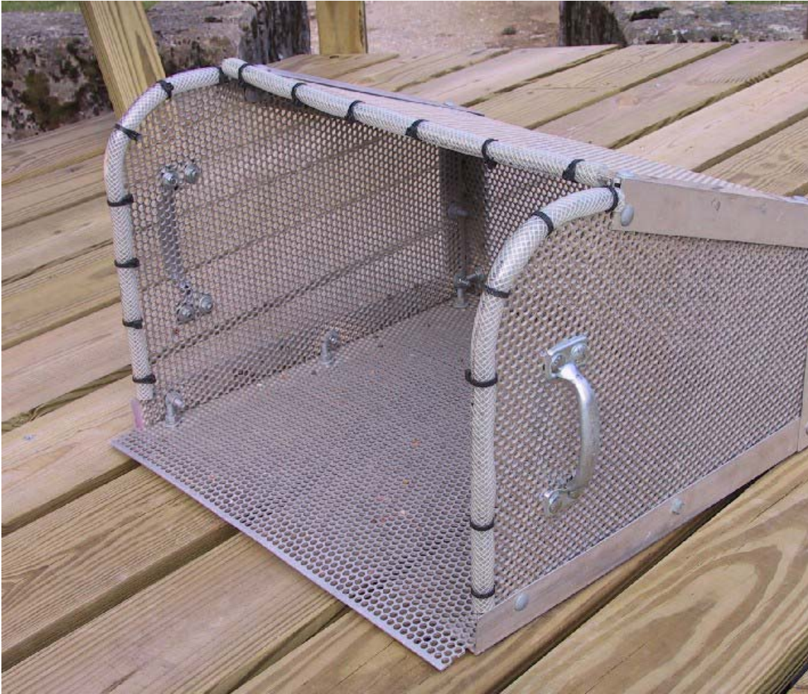
Figure 5. The Ferraro streambed sampler. This sampler is made with perforated aluminum and was designed to hold all substrate excavated from a 0.25 m 2 quadrat.
