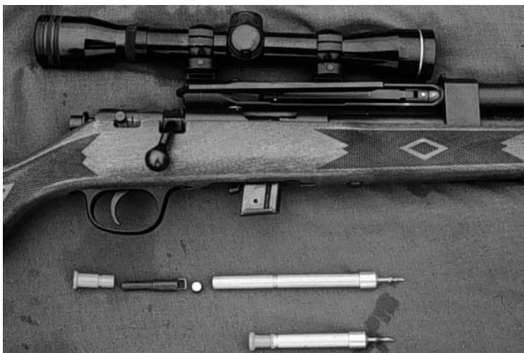
Figure 20. Dart rifle used for delivery of antifertility agents, vaccines, and immobilizing drugs
